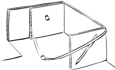
11. Fold the rectangular scrap (about 7 cm by 6 cm) in half the long way over the edge of the base where the shading is on the pattern. Staple it in place with four or five staples. Make sure there is room to slide a nail into the fold.
