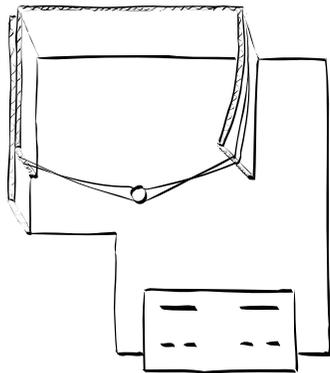
12. Unbend a regular paper clip as illustrated. Put a paper fastener in one switch hole, and secure the paper-clip switch in position with the other paper fastener.
